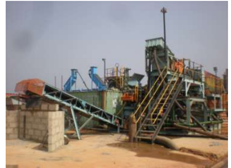
Operational 5tph DMS plant
