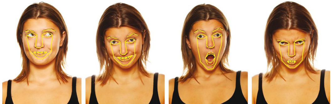
These stills taken from a video sequence illustrate a small portion of faceAPI's face tracking functionality. The wire-frame overlay portrays faceAPI's real-time determination of the changing location, orientation and shape of the subject's face and head. These parameters provide the raw data needed by many applications and devices to engage with, respond to or otherwise be aware of various interactions with a real person. Consequently as an enabling technology the faceAPI is at the forefront of the next generation of human aware interfaces and devices.
