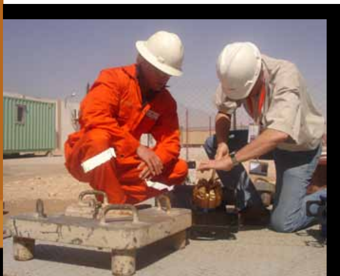
Re-dressing a drill bit for the Algerian drilling campaign.
