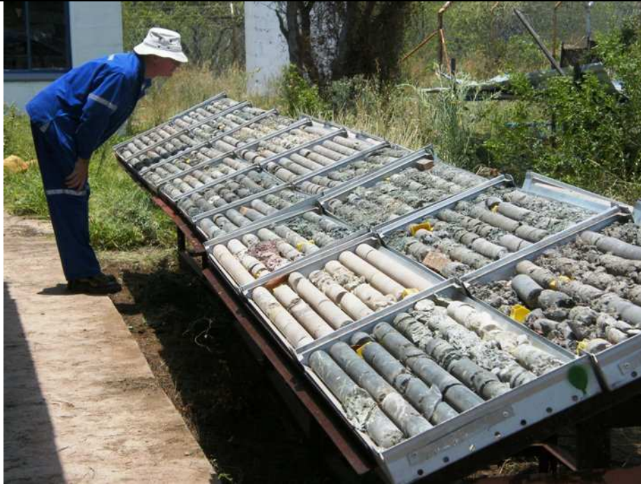
Figure 11-2 Core logging during the site visit conducted for this report
