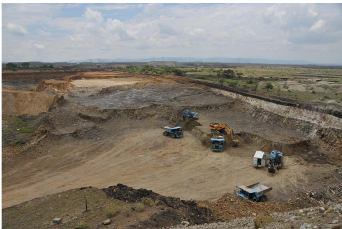
Exhibit 7: Relatively shallow dipping chromite reefs facilitate a simple opencast operation
