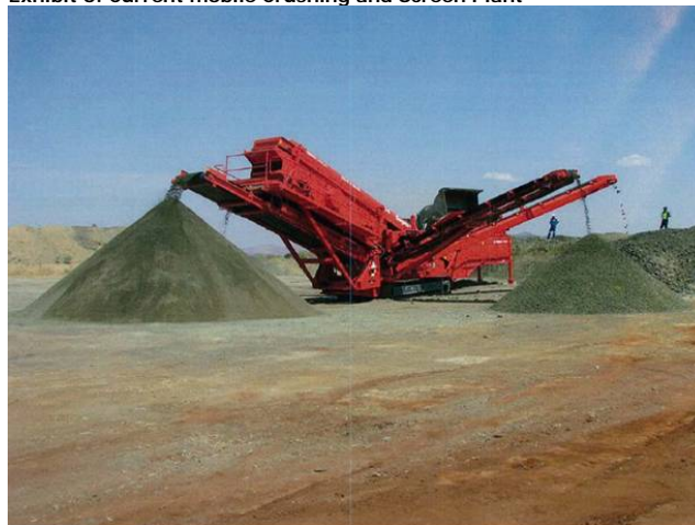
Exhibit 6: Current mobile Crushing and Screen Plant
